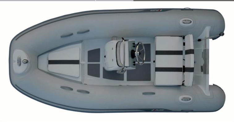
**Overal Length** : 11'6"/3.50m Number of Chambers : 3 Shaft Length : 20" / 50.8cm **Overal Beam Person Capacity** : 5 RDC Design Category : C : 5'7"/1.70m Inside Length : 8'6"/2.60m Weight : 284lb / 129kg Inside Beam Recommended HP : 2'8"/ 0.81m : 15hp / 11.2kw **Tube Diameter** : 17"/ 0.43m Maximum HP : 20hp / 14.9kw
